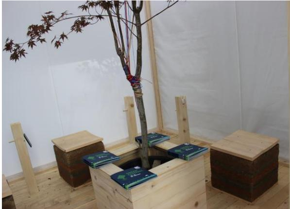
Multifunctional structure: Solar phone charging station and reading corner with rammed earth seats. Constructed by Blerim Lutolli and Argjira Krasniqi.
