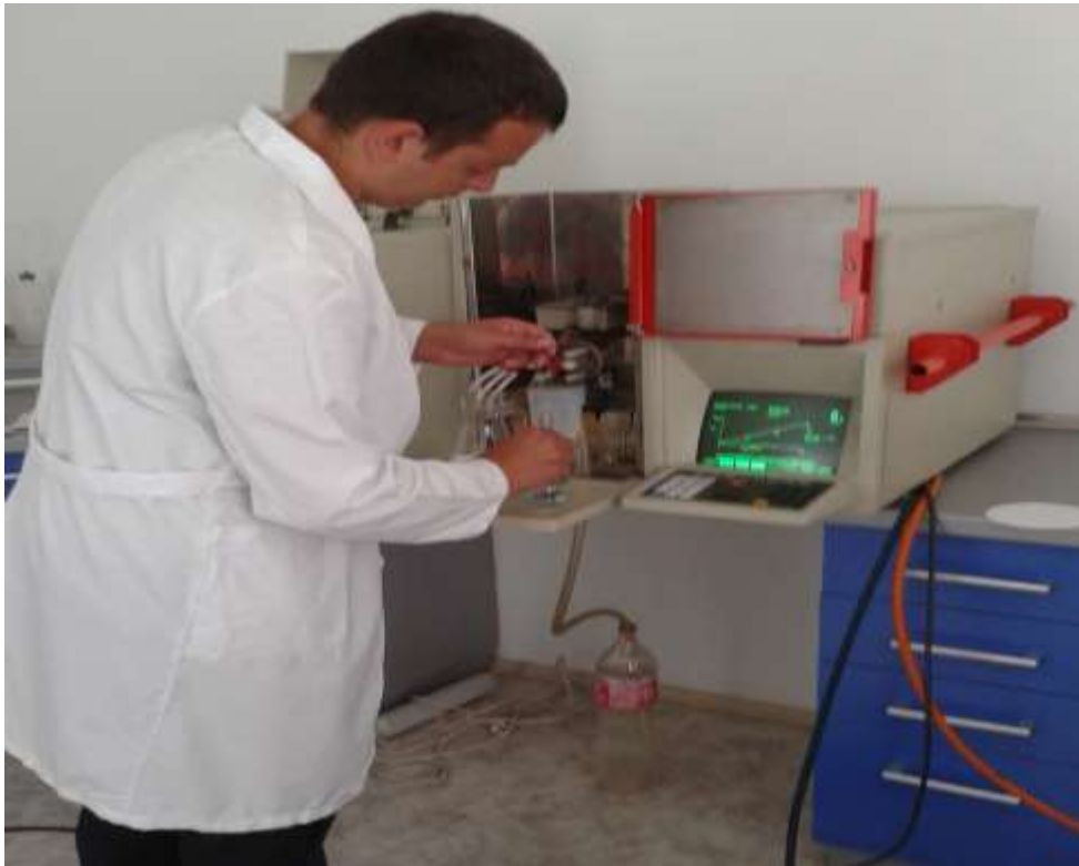
Picture 8. Determining heavy metals (AAS spectroscopy)
