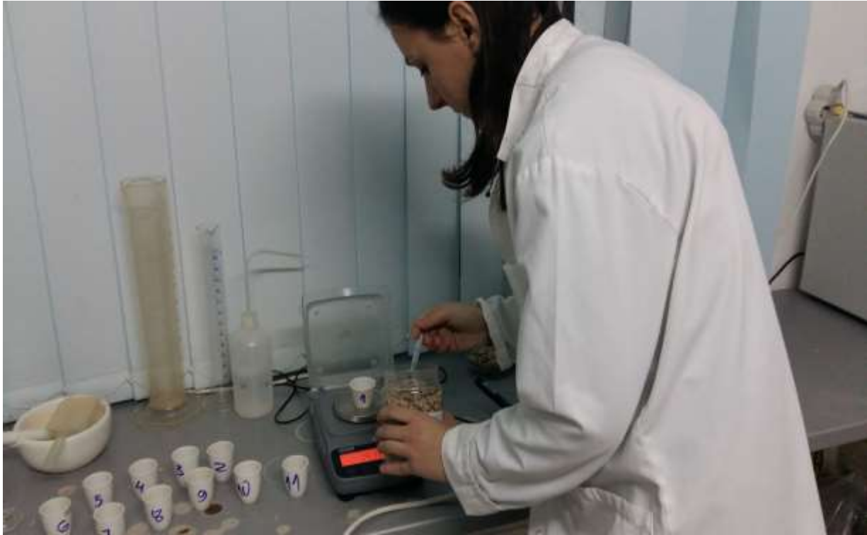
Picture 4. Measuring samples for determining ash content
