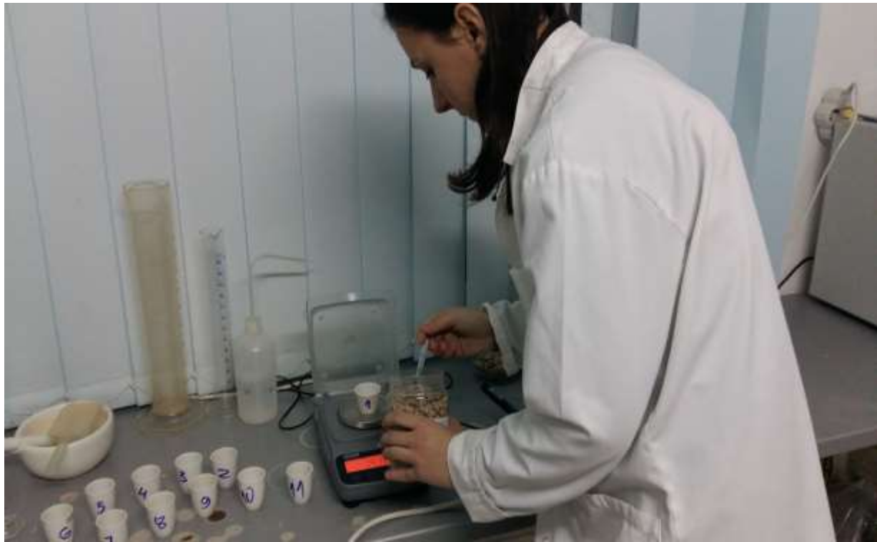
Picture 4. Measuring samples for determining ash content
