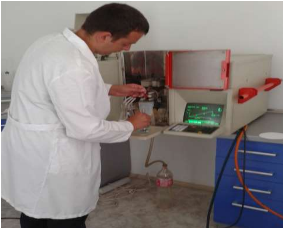
Picture 8. Determining heavy metals (AAS spectroscopy)
