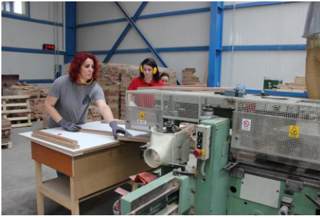
Women employees making finger joint planks at Dijamant wood processing factory.
